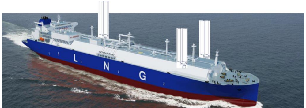
Graphical rendering of the LNG carrier concept with DFE+-WAPS setup
